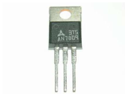
Figure 4: The 7809-voltage regulator [9]
