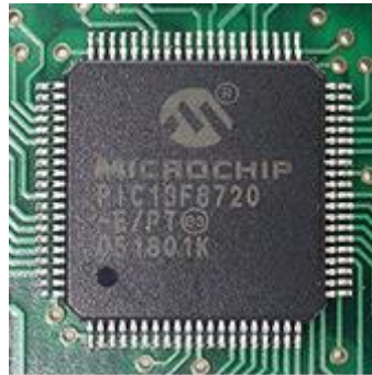
Figure 7: A microcontroller (PIC18F8720 from Microchip) on board. [9]
