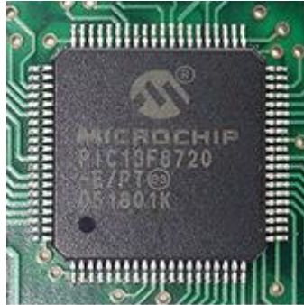
Figure 7: A microcontroller (PIC18F8720 from Microchip) on board. [9]
