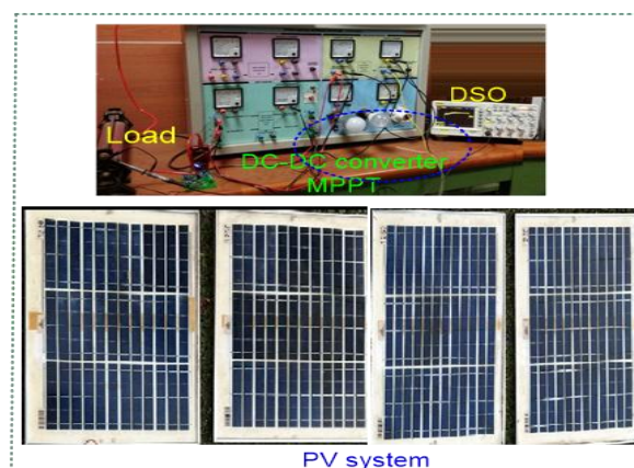
Figure 17: Experimental setup for MPPT-assisted PV system
