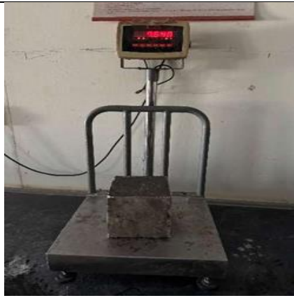
Figure 10: Water absorption test
