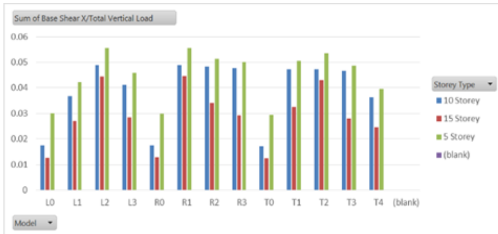
Figure 12: Graph showing comparison of base shear to seismic weight ratio for various models with shear wall
