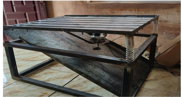
Figure 2: Fabricated and assembled sand sieving machine
