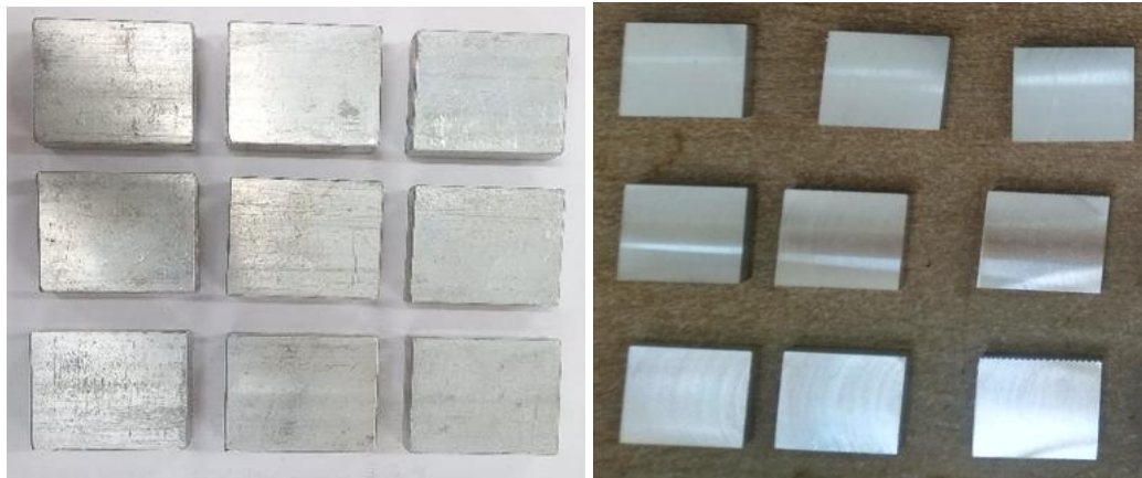
Figure 3: Specimen of Al-6061 alloy (a) Before machining and (b) After machining
