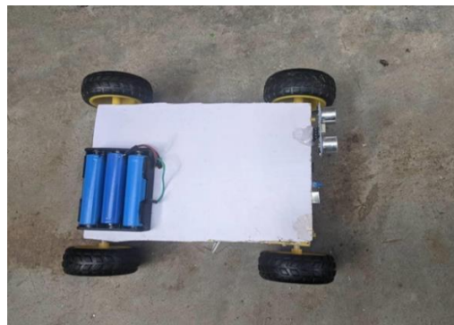
Figure 3: Hardware prototype of the proposed four-wheeled mobile robot
