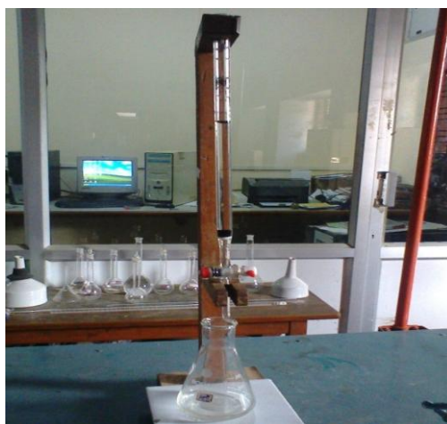
Figure 2: Ion exchange column for ion exchange experiment
